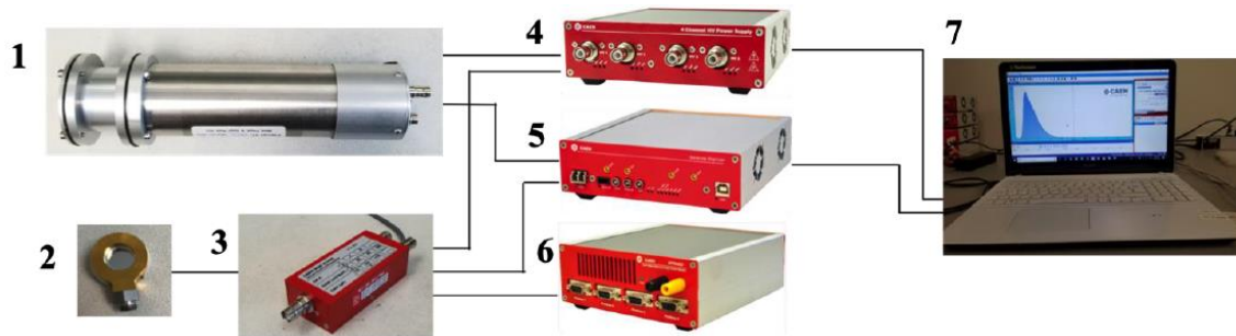
Figure 2.1 Beta-ray spectrometers system. Labeled component: 1 Plastic scintillator detector, 2 Silicon SBD detector, 3 Charge sensitive preamplifier, 4 High voltage supply, 5 Digital pulse processor, 6 Preamplifier power supply, 7 Data acquisition laptop
