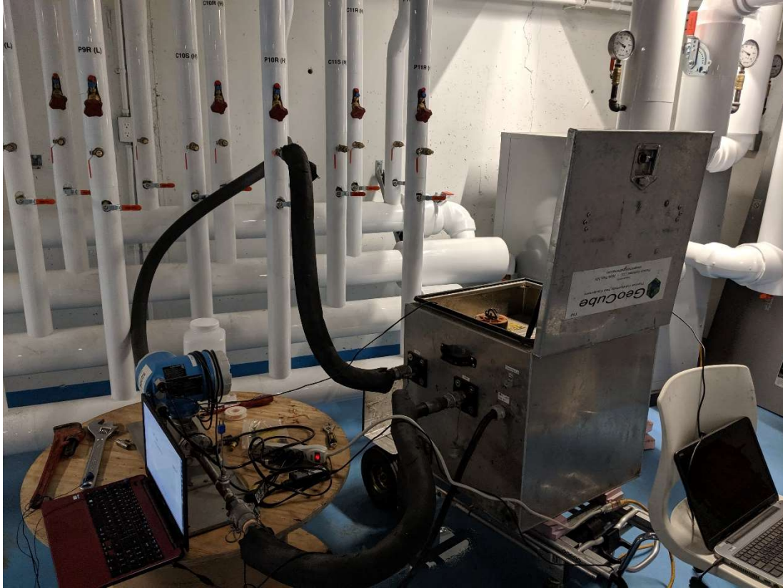
Figure 3.8 - GeoCube and Flowmeter during TRT
