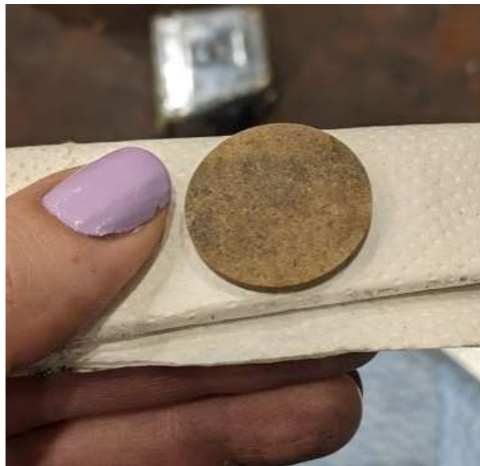
Figure 5.16 - Compressed Soil Sample (1 Inch Diameter) Used for LFA Testing
