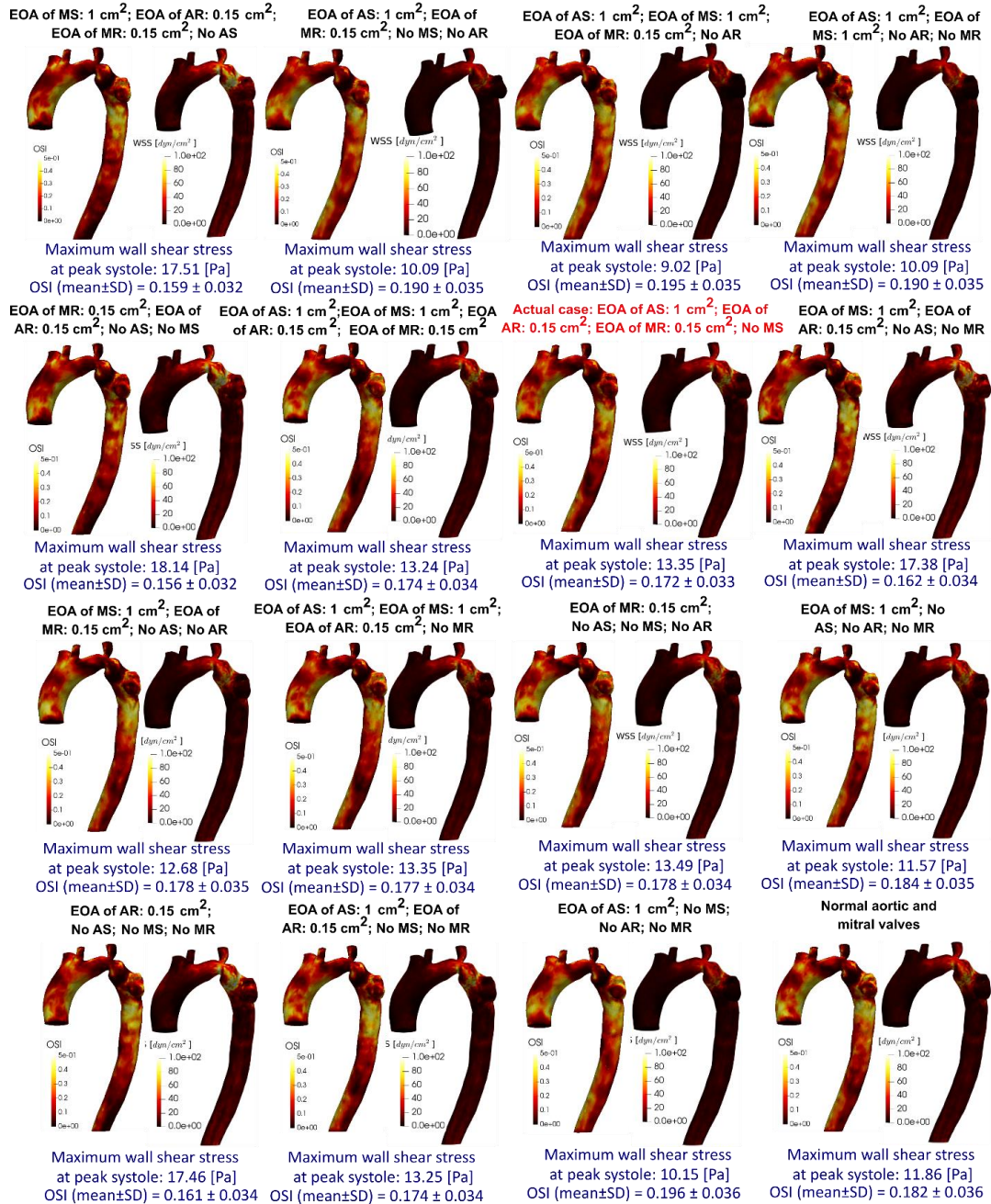
Figure 3-6. Flow modeling in Patient No. 1. Computed wall shear stress (WSS) and Oscillatory shear index (OSI) using the computational framework (based on LPM and LBM) in sample Patient No. 1 (Actual patient in red text in this figure). OSI can be computed as OSI = \frac{1}{2} \left( 1 - \frac{\int_0^T \tau dt}{\int_0^T |\tau| dt} \right) . Here, T and \tau are the cardiac cycle period and instantaneous wall shear stress, respectively.
