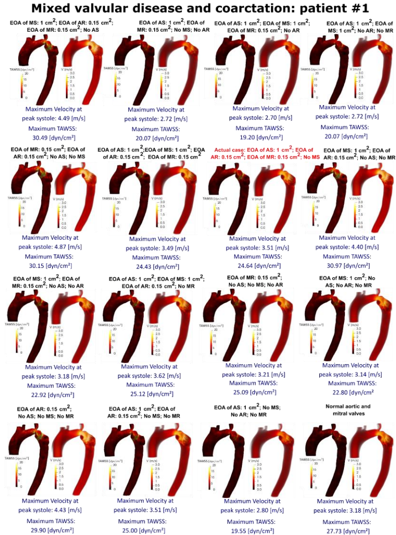
Figure 4-4. Flow modeling (local) in Patient No. 1. Computed velocity magnitude and time-averaged wall shear stress (TAWSS) using the computational framework (Lattice Boltzmann method and lumped parameter model) in sample Patient No. 1. Actual patient (in red font in this figure) has severe aortic stenosis ( EOA_{AS}=1 \text{ cm}^2 ), moderate aortic valve regurgitation ( EOA_{AR}=0.15 \text{ cm}^2 ), moderate mitral valve regurgitation ( EOA_{MR}=0.15 \text{ cm}^2 ) with no mitral stenosis. This patient has brachial pressures of 70 and 125 mmHg, forward LV stroke volume of 110 mL, maximum LV pressure of 170 mmHg and LV workload of 2.4923 J. The total shear stress exerted on the wall throughout the cardiac cycle was evaluated using the time-averaged wall shear stress (TAWSS) which is obtained as TAWSS = \frac{1}{T} \int_0^T |\tau| dt . Here, T and \tau are the cardiac cycle period and instantaneous wall shear stress, respectively.
