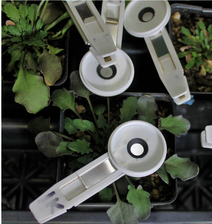
Figure 2.1: Detachable leaf clips on expanded leaves of a Yukon Eutrema plant for OJIP measurements. During dark adaptation a metal tab in the window of the clip is set in a closed position and for measurements the tab slides away to expose the leaf to light.
