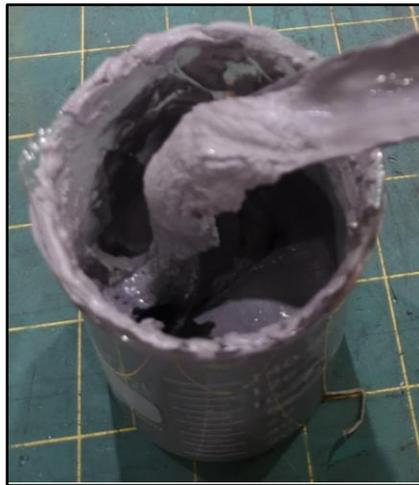
**Figure 24: Aluminum paste (Al powder + liquid coolant)**
