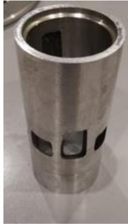
**Figure 47: Workpiece preparation after water jetting, and turning the outer surface**
