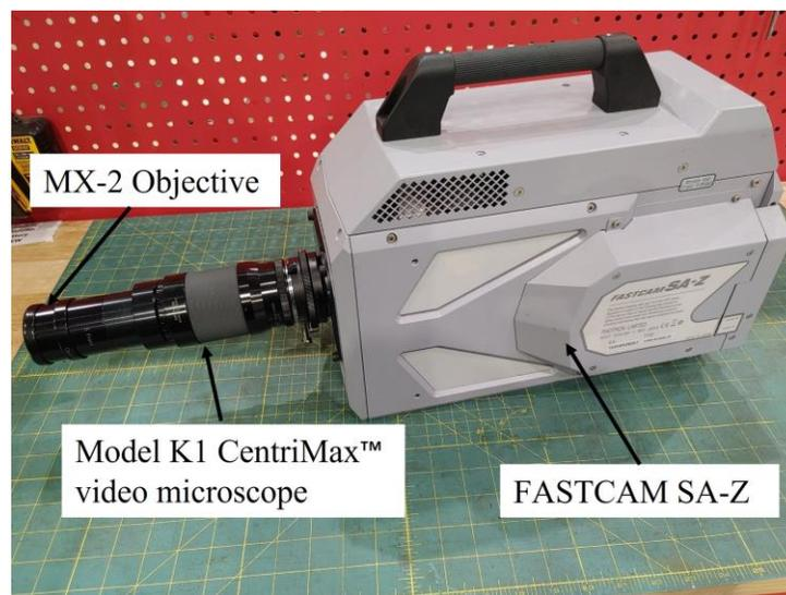
Figure 49: High-speed camera
