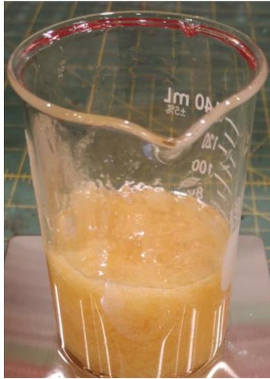
**Figure 25: High viscosity coolant**
