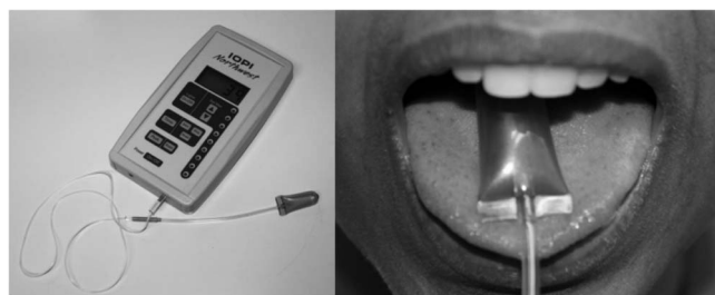
Figure 1. The Iowa Oral Performance Instrument (IOPI), a handheld device that measures tongue pressure, is depicted on the left, and the anterior placement of an IOPI tongue pressure bulb is depicted on the right.
