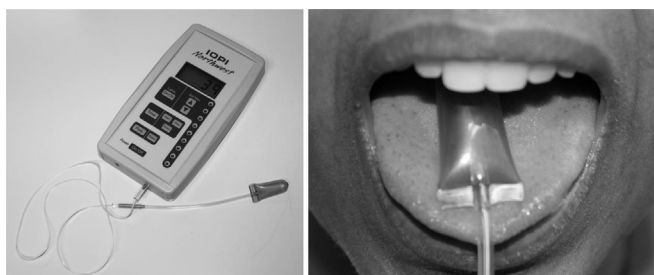
Fig. 1. The Iowa Oral Performance Instrument (IOPI), a hand-held device to measure tongue pressures is depicted on the left, and the anterior placement of an IOPI tongue pressure bulb is depicted on the right.
