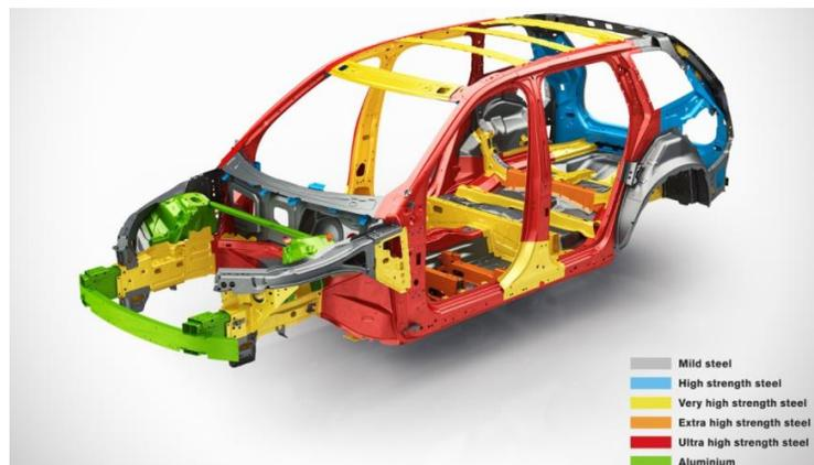
Figure 1.1: The 2013 Honda Accord BIW containing 51% AHSS [5].
