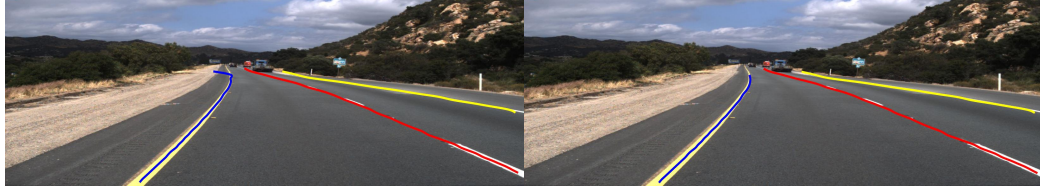
(a) Lane interpolation after adding dice loss (b) Lane interpolation after removing outliers
