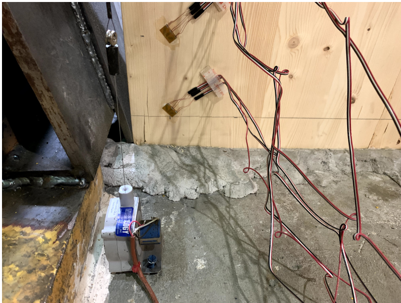
Figure 5.2: Compression Toe at 1.5% Drift
