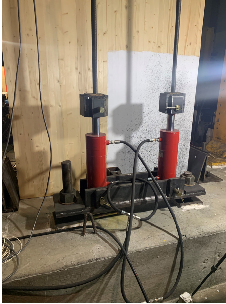
(a) 250kN Capacity Actuators at Base of the Wall
