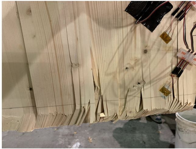
Figure 5.6: Decompression Toe at 4% Drift
