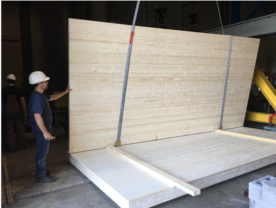
Figure 4.1: CLT Panel Manufactured by [Element5, 2019]
