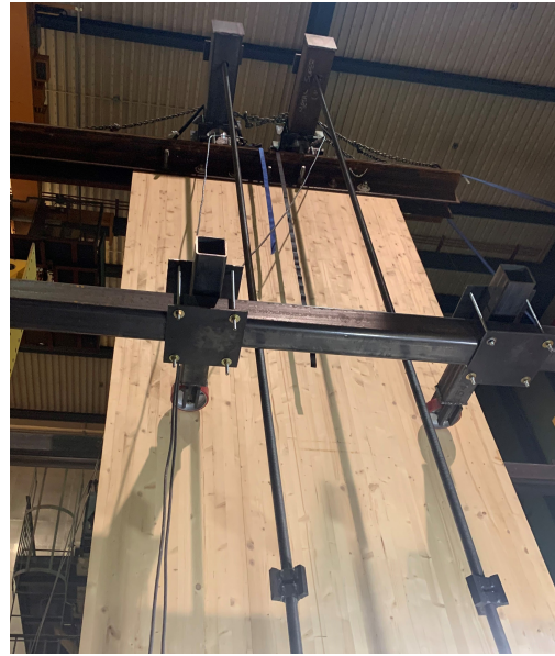
(b) Threaded Tensioning Rods Connecting Actuator to Loading Beam
