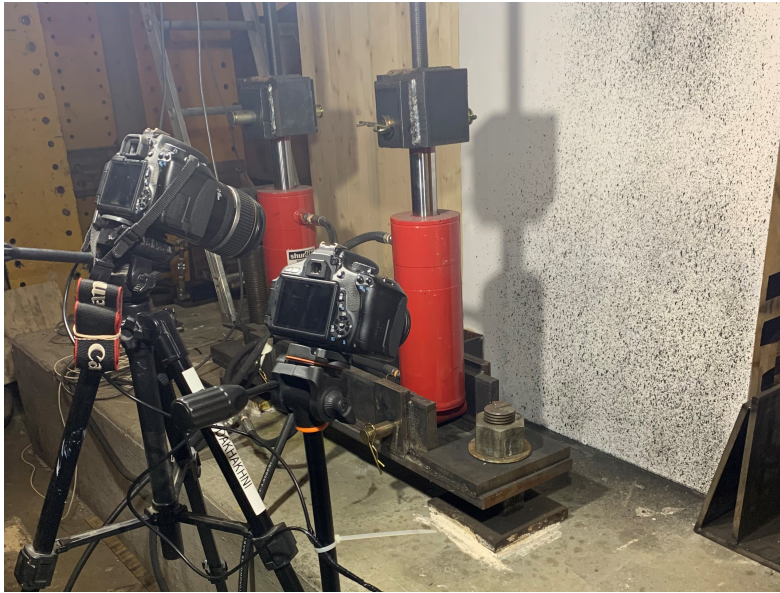
Figure 4.6: Digital Image Correlation Setup
