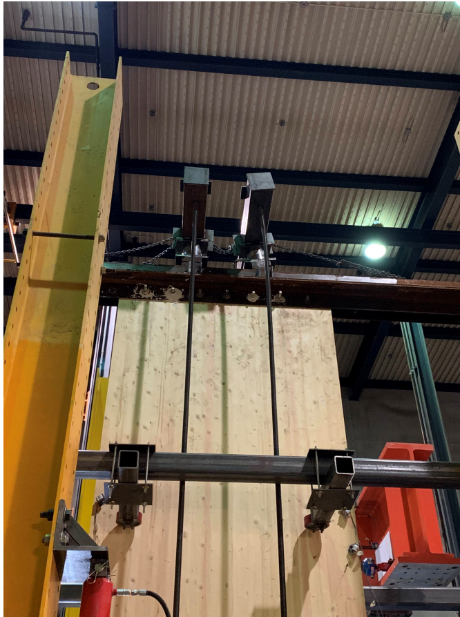
Figure 5.10: Axial Load Distribution Beam during 2.0% Drift Cycle
