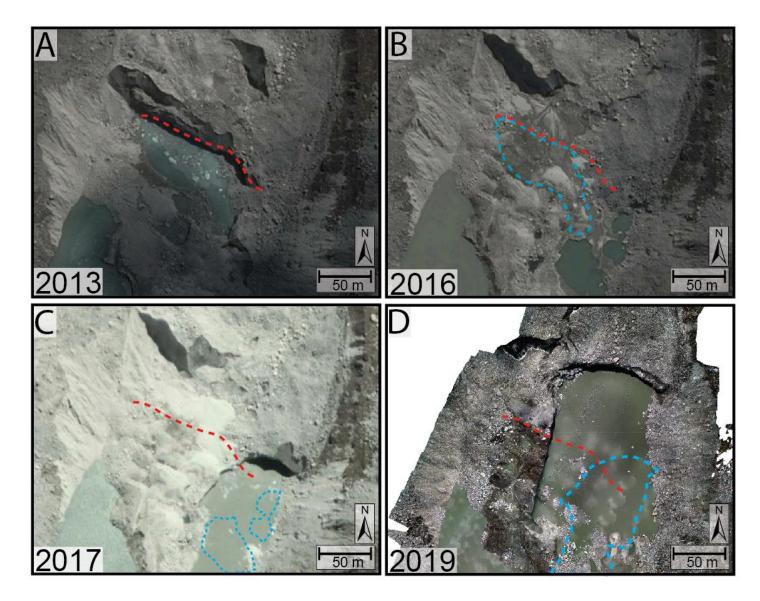
Figure 3.10: Moraine slope failures occur along the inner side of the latero-frontal moraine and transport sediment into the lake. A moraine slope failure that occurred at some time between 2013 (A) and 2016 (B) is recorded by satellite images taken in 2016 (red arrow; Google Earth, 2013, 2016).
