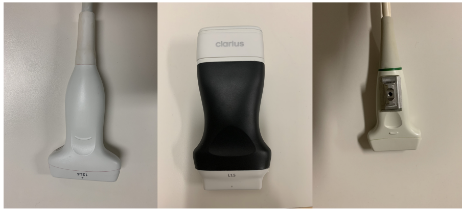
Figure 2.3: Ultrasound Probes. From left to right, Siemens S3000 12L4, Clarius L15, SonixTouch L14-5. These particular examples are all linear phased array that produce 2D images.
