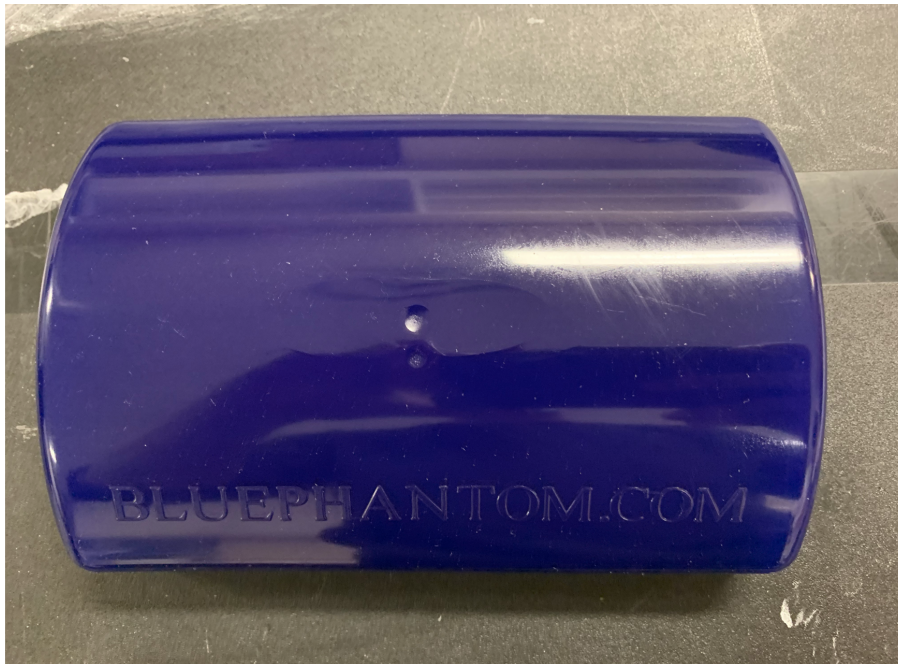
Figure 3.2: Soft tissue mimicking BLUE phantom from CAE Healthcare (Sarasota, FL).
