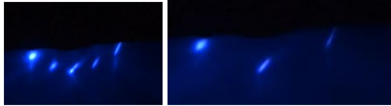
Figure 2.17: RHEED patterns for GaAs(111)A homoepitaxial growth, which will be elaborated upon in chapter 3. A 2 \times 2 reconstruction, meaning the periodicity of the surface is twice the bulk, is shown on the left and a (1 \times 1) pattern implying a surface reconstruction (during Bi deposition on GaAs(111) with identical surface periodicity to the bulk is shown on the right.
