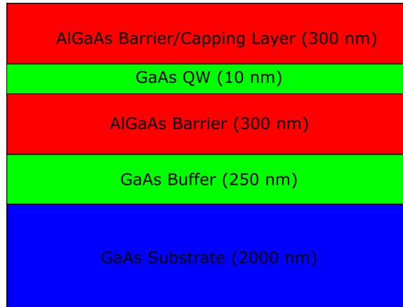
Figure 5.2: Schematic of simulated QW using Nanohub 1D Schrödinger–Poisson solver tool.
