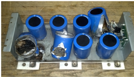
(c) Capacitor explosion caused by electrolyte evaporation
