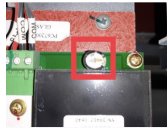
(b) An Exploded Capacitor on a PCB
