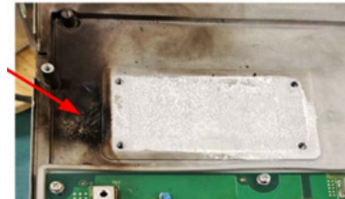
(d) Burns on Heat Sink due to Flashovers
