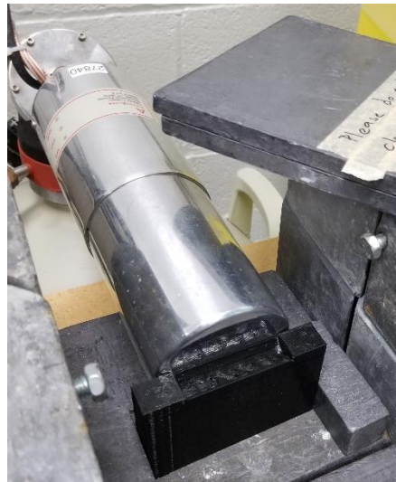
Figure 18: Close-up of the detector configuration during data collection. The 3D-printed plastic component used to mount the sample-containing vials is seen in black, at the bottom. Also visible are the lead blocks used to shield the apparatus.
