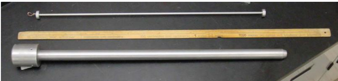
Figure 14: Image of a wire holder (top) and a sample holder (bottom) used during irradiation procedures [41]. A meter stick is shown between these two pieces of equipment, for scale.
