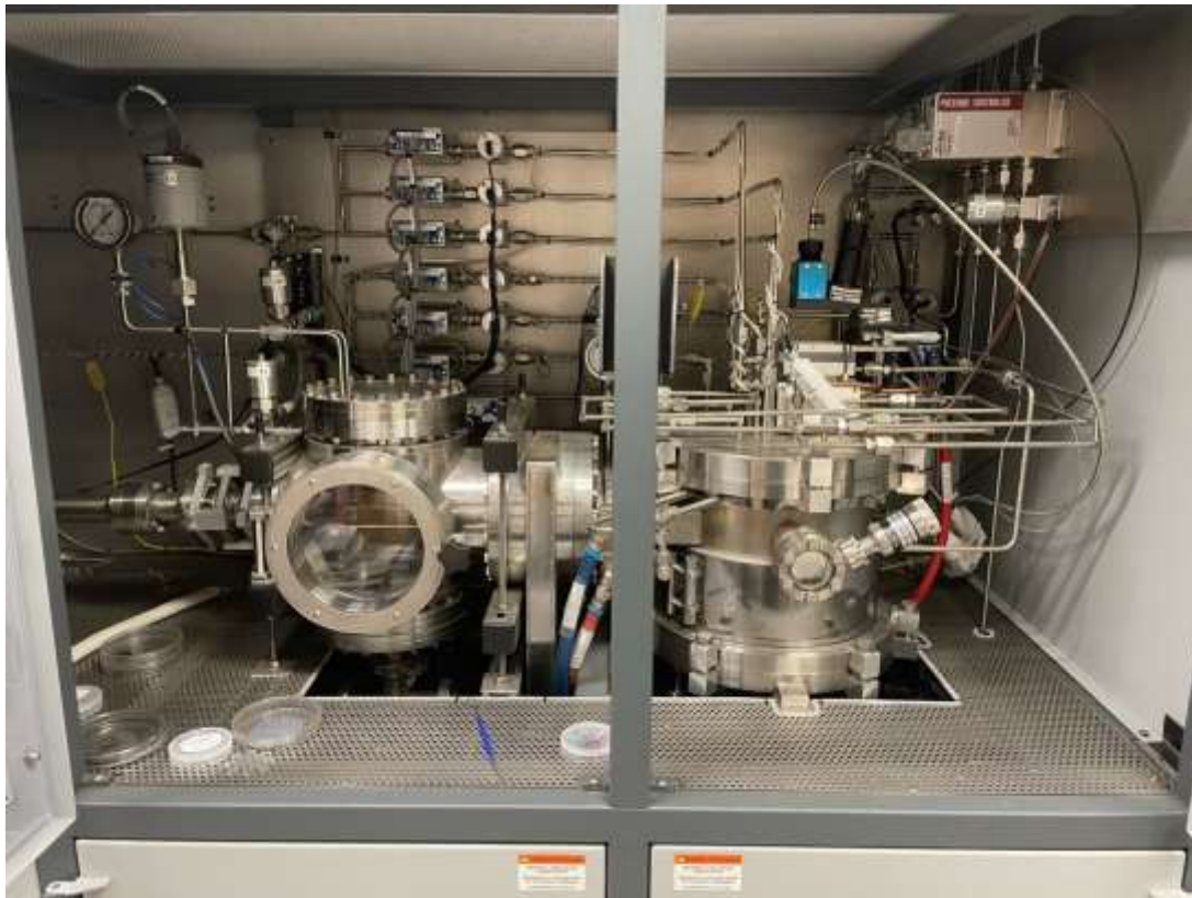
Figure 15: McMaster University MOCVD Chamber
