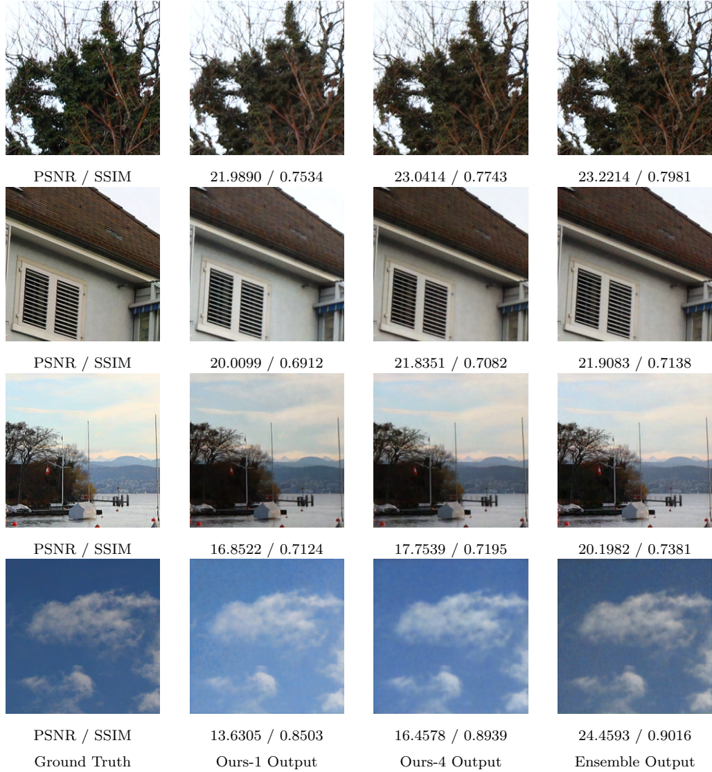
FIGURE 4.1: PSNR/SSIM and visual comparisons of reconstructed images from different network models. Ours-4 and Ours-1 denote our demosaiced and RAW models, respectively.
