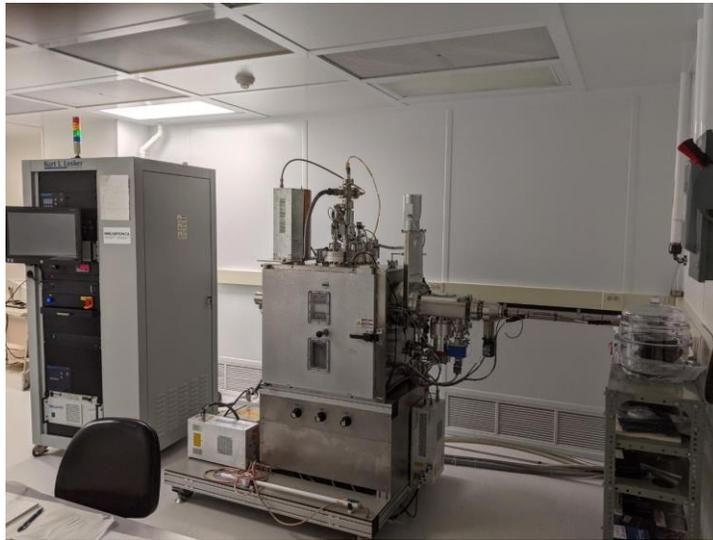
**Fig. 2.1.** Picture of Kurt J. Lesker PVD Pro 200 thin film deposition system in the CEDT cleanroom, with control tower on the left and vacuum chamber on the right.
