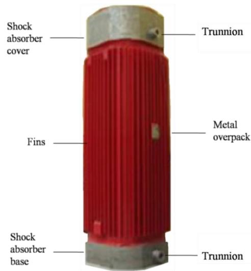
**Fig. 2.7** CASTOR Ic- DIORIT Dry Cask for SNF transport and storage, adapted from (Droste, 2013)
