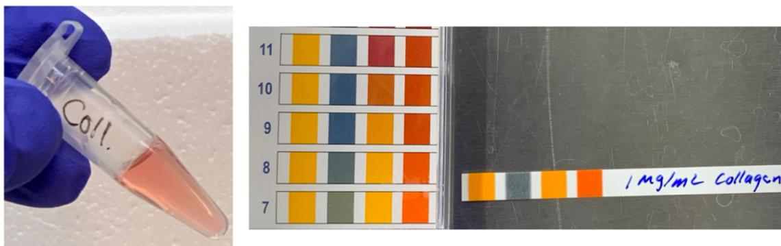
**Figure 12.** 1 mg/mL collagen prepared by neutralization of acid-solubilized concentrated rat-tail collagen type I. pH indicator dye phenol red turns pale pink-orange indicating a near physiological pH (~ 7.4). pH test strip results also estimate a pH between 7 and 8.
