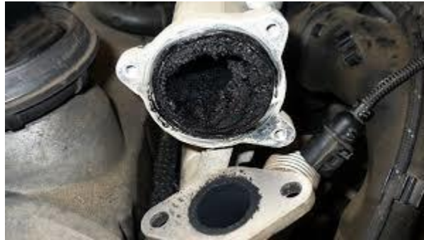
Figure 1.6 Clogged EGR valve
