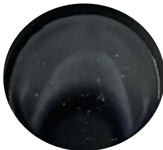
Figure 6.S7. Picture of the biofouled membrane after 18 h filtration of E. Coli suspension with a concentration of 1 \times 10^7 CFU/mL.
