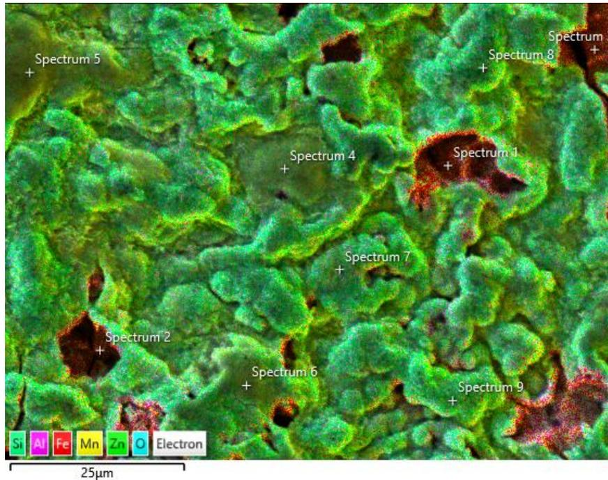
Figure 5.9: EDS map of wall of galvanized DHPF 2.5%Mn austenitized for 180 s.
