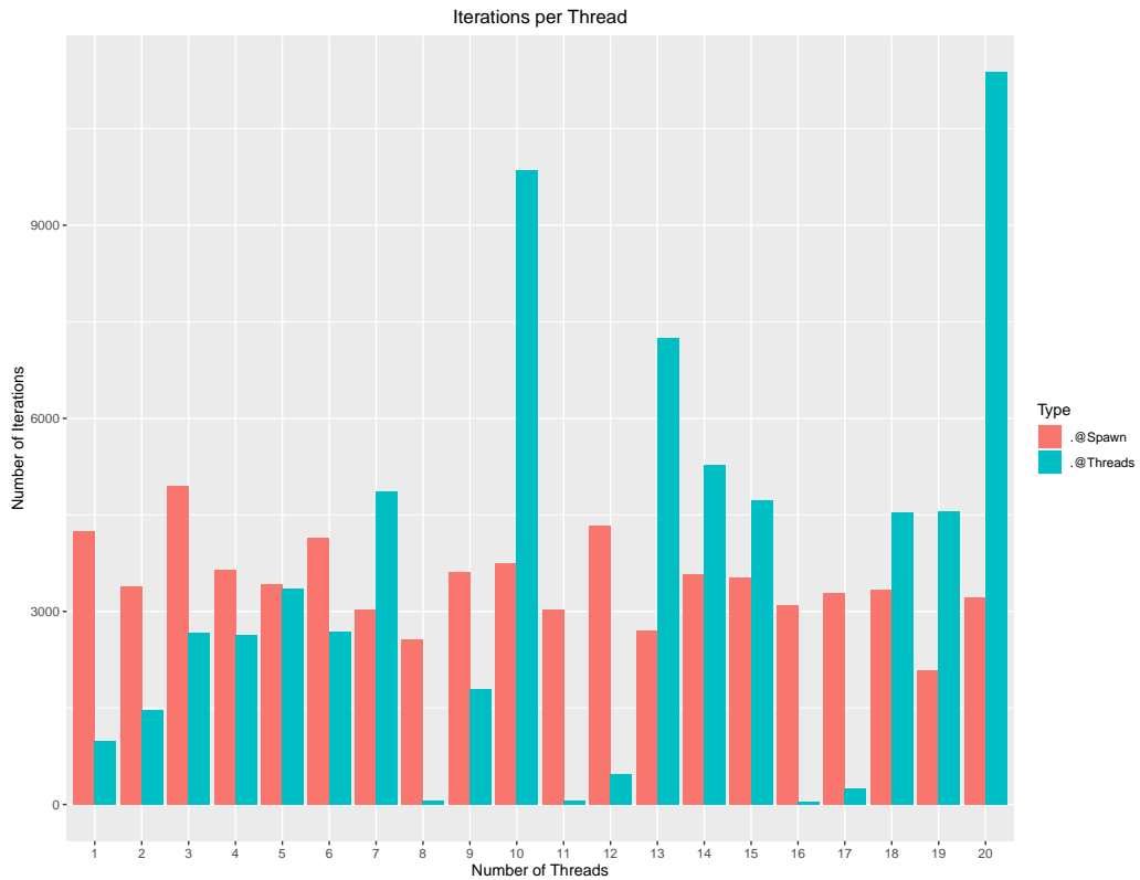
Figure 4.1: Iterations per thread using different base multithreading implementations in Julia.
