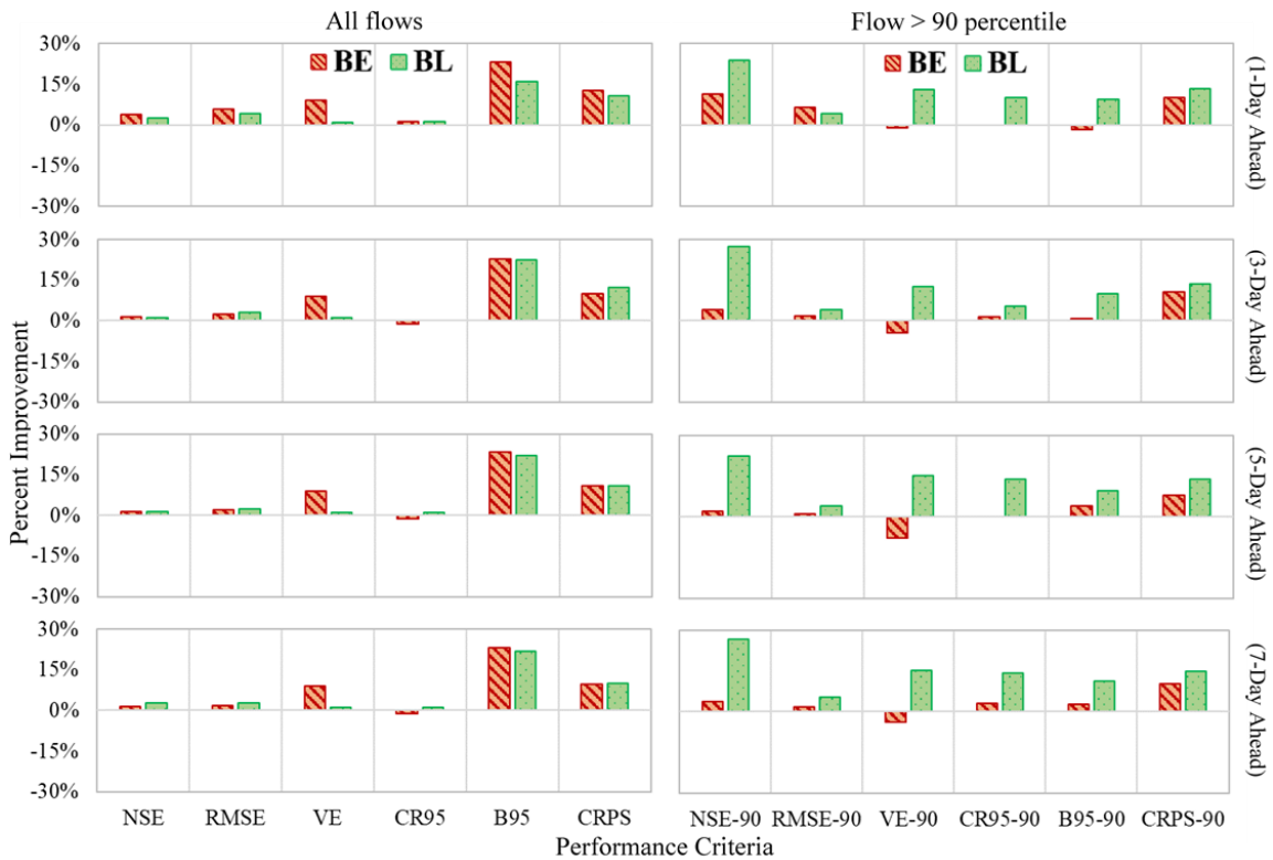
Figure 4-8 The percent improvement of different performance statistics in both Big East River and Black River watersheds. The positive value of percent improvement shows the positive effect of utilizing E-35 in comparison to E-7
