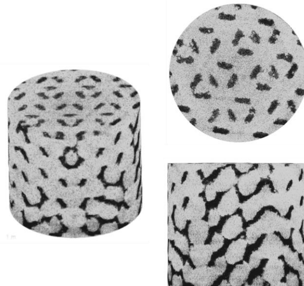
Figure 2: Cylindrical volume ( h = 7 mm, \varnothing = 8 mm) extracted from the micro-CT reconstruction of an as-fabricated stainless steel scaffold. Pores (darker regions) in the stainless steel (lighter regions) appear ellipsoidal in cross-section as a result of the 45^\circ unit cell tilt. Junctions between these pores are visible around the periphery of the cylindrical volume.
