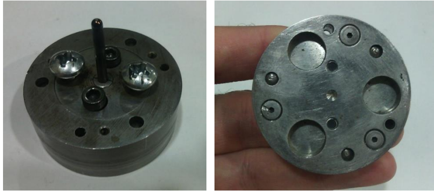
Figure 12: New collet designed for the MMRI Tribometer (Mark III)
