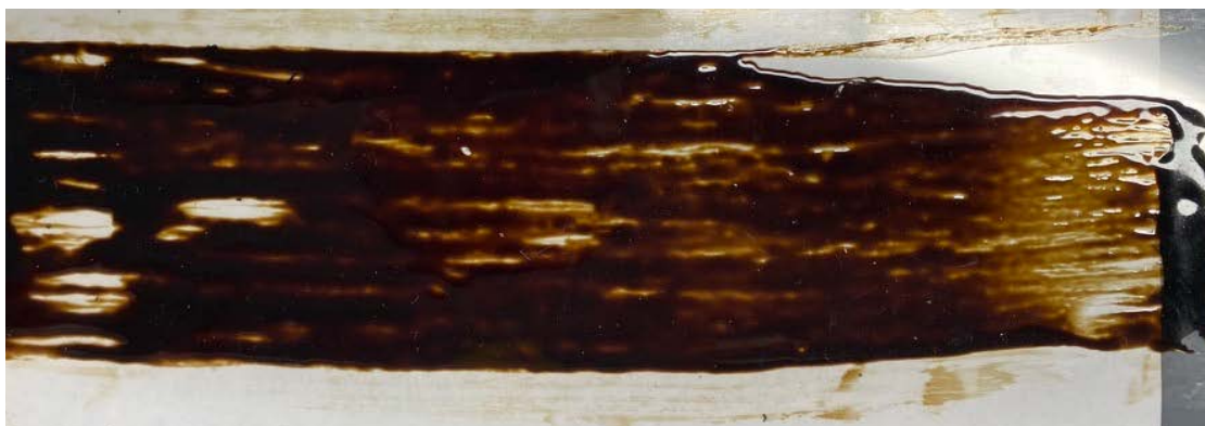
Figure 6.63: Poor quality H-A-N 1:1 elastomer film cast with higher viscosity oils.
