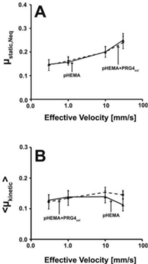
**FIGURE 3.** Effect of PRG4 on boundary lubrication at a human cornea-pHEMA biointerface. Static,  $\mu_{static}$  (A), and kinetic,  $\mu_{kinetic}$  (B). Friction coefficients measured in baths of saline and PRG4 at 300  $\mu\text{g}/\text{mL}$  in saline. Values are mean  $\pm$  SEM ( $n = 6$  cornea,  $n = 6$  eyelid) with an average normal stress of  $21.3 \pm 0.6$  Pa for cornea. Lubricant effect ( $p = 0.99$  A;  $p = 0.69$ ), velocity effect ( $p < 0.01$  A; B  $p = 0.86$ ).
