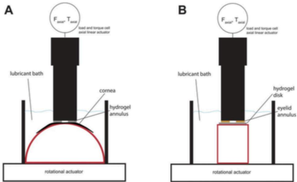
FIGURE 1. Schematic of the *in vitro* human cornea-hydrogel (A) and human eyelid-hydrogel (B) biomechanical friction test setup.
