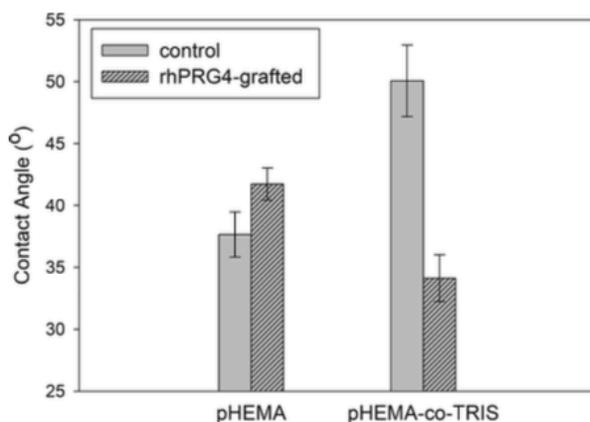
**Figure 3.** Impact of surface rhPRG4-grafted on the surface wettability. The static water contact angles ( $\pm$ SD) of unmodified (control) and rhPRG4-grafted pHEMA and pHEMA-co-TRIS hydrogel surfaces, swollen in Milli-Q water, using the captive bubble technique ( $n = 6$ ).
