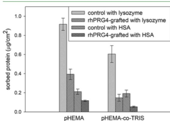
**Figure 4.** Impact of surface rhPRG4-grafted on protein deposition. The amount ( $\pm$ SD) of physisorbed lysozyme and human serum albumin (HSA) on the surface of unmodified (control) and rhPRG4-grafted pHEMA and pHEMA-co-TRIS hydrogels upon a 6 h incubation period at room temperature ( $n = 6$ ).
