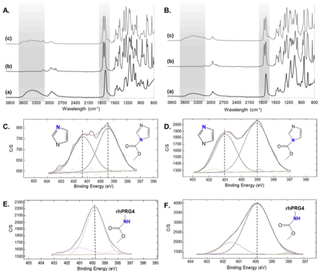
**Figure 1.** Characterization of surface chemistry. ATR-FTIR adsorption spectra of (A) pHEMA and (B) pHEMA-co-TRIS for (a) unmodified (control), (b) CDI-activated, and (c) rhPRG4-grafted hydrogel surfaces (600–4000  $\text{cm}^{-1}$ ). High-resolution  $\text{N}_{1s}$  XPS spectra for (C, D) CDI-activated and (E, F) rhPRG4-grafted pHEMA and pHEMA-co-TRIS hydrogel surfaces, respectively (395–405 eV).
