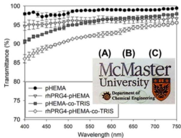
**Figure 6.** Impact of surface modification on optical transparency. Transmittance spectrum ( $\pm$ SD) for the unmodified (control) and rhPRG4-grafted pHEMA and pHEMA-co-TRIS hydrogel disks ( $n = 6$ ). Inset: a photograph of (A) unmodified, (B) CDI-activated and (C) rhPRG4-grafted pHEMA (top) and pHEMA-co-TRIS (bottom) hydrogel materials.
