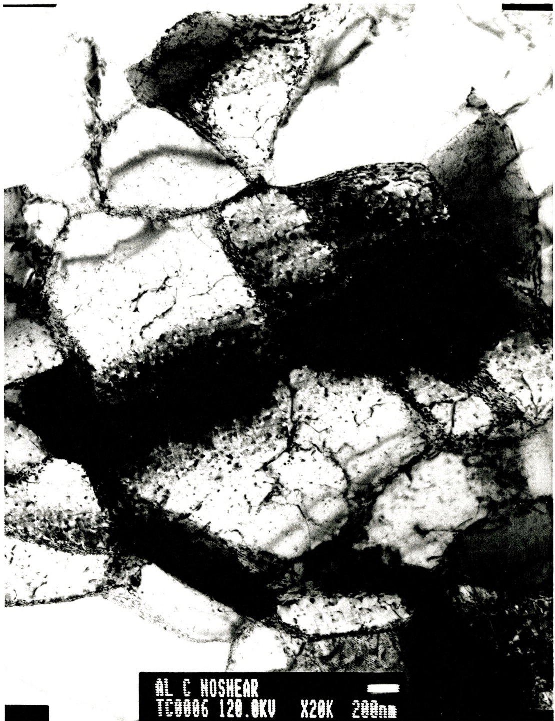
Figure 3.44/ TEM micrograph of Al-0.4%Cu deformed to a true strain of 1 at room temperature, region free of shear bands
