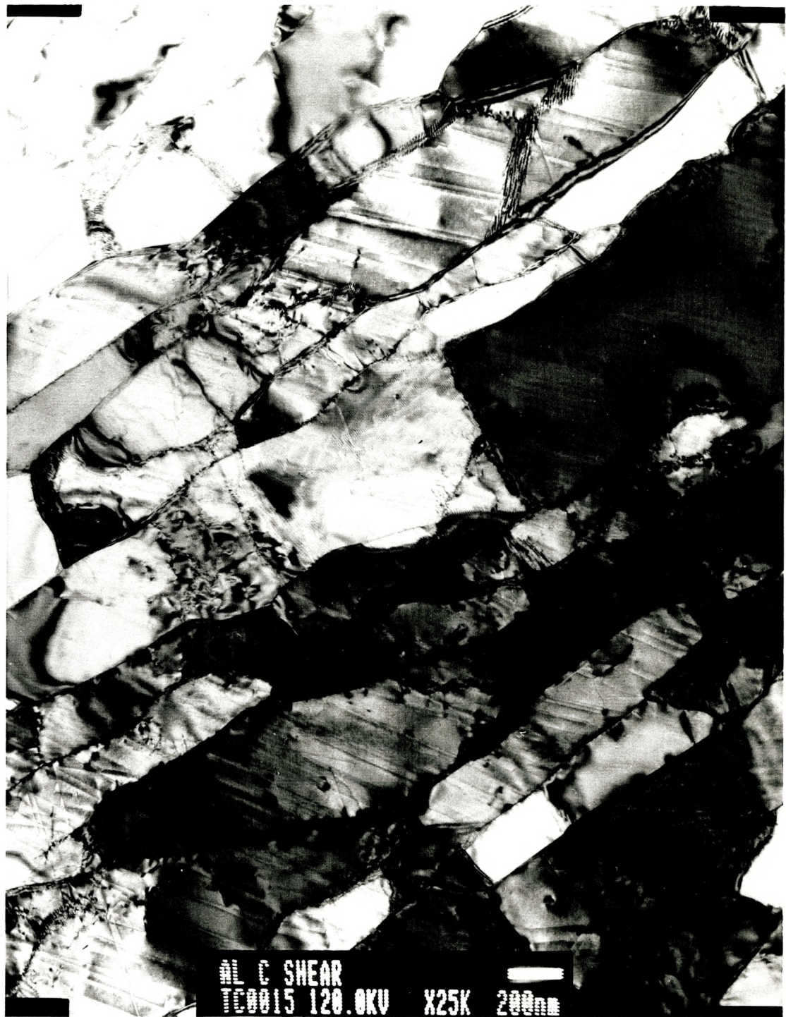
Figure 3.43/ TEM micrograph of Al-0.4%Cu deformed to a true strain of 1 at room temperature, shear banded region
