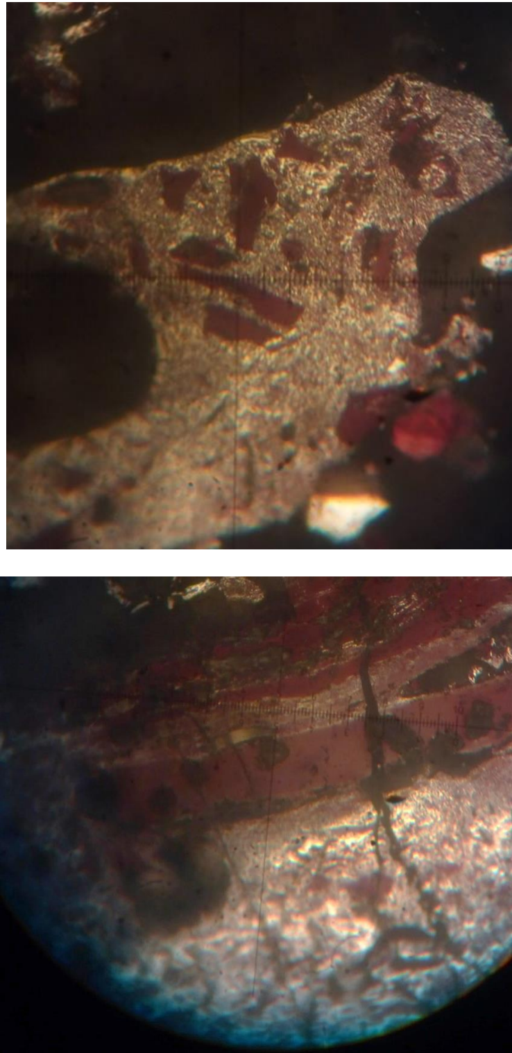
Figure 5-13 – Solid Base Blend Coke Structure (Top) Fissure Through Biomaterial and Coke Structure (Bottom)
