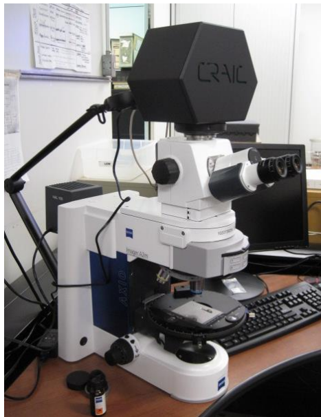
Figure 4-2 - Optical Light Microscope with Polarized Light Source, Rotating Stage and Photomultiplier (manual or automatic) for Coal Petrography at Canmet
