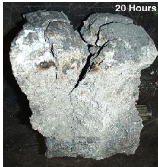
Figure 2-16 - Visible fissure in the fully coked piece (Jenkins, Mahoney, & Keating, 2010b)
