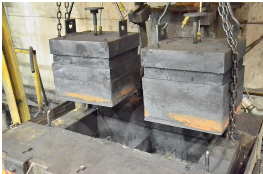
Figure 4-5 - SHO duplicate chamber design at Canmet
