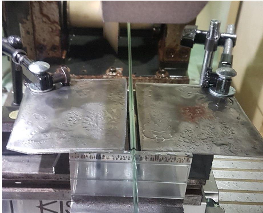
Figure 3.6: Jet positioned above target for hydrodynamic pressure test, with floating guards to prevent signal contamination from spray
