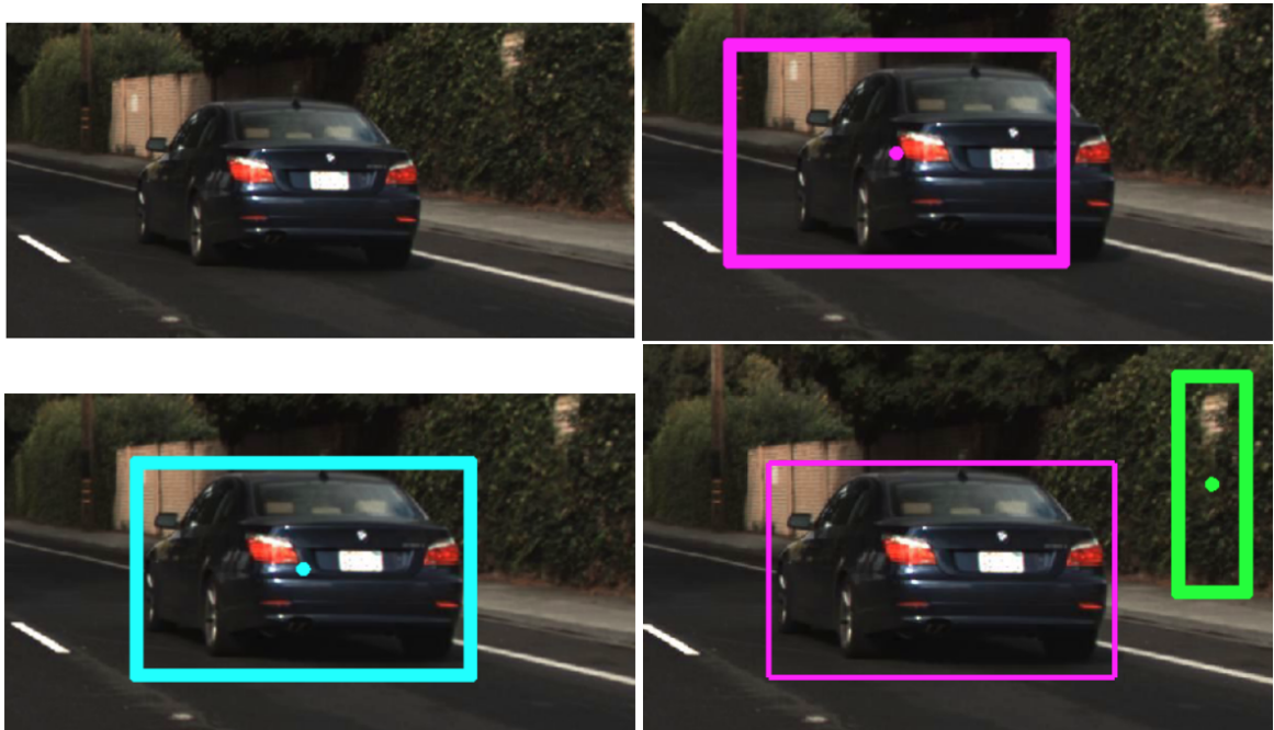
Figure 1.7: From the top, the first image is a missed detection. The second is an incorrect localization, the third is an incorrect classification, and the fourth is a false alarm. A purple bounding box corresponds to a car. A green bounding box corresponds to a pedestrian. A blue bounding box corresponds to a truck.
