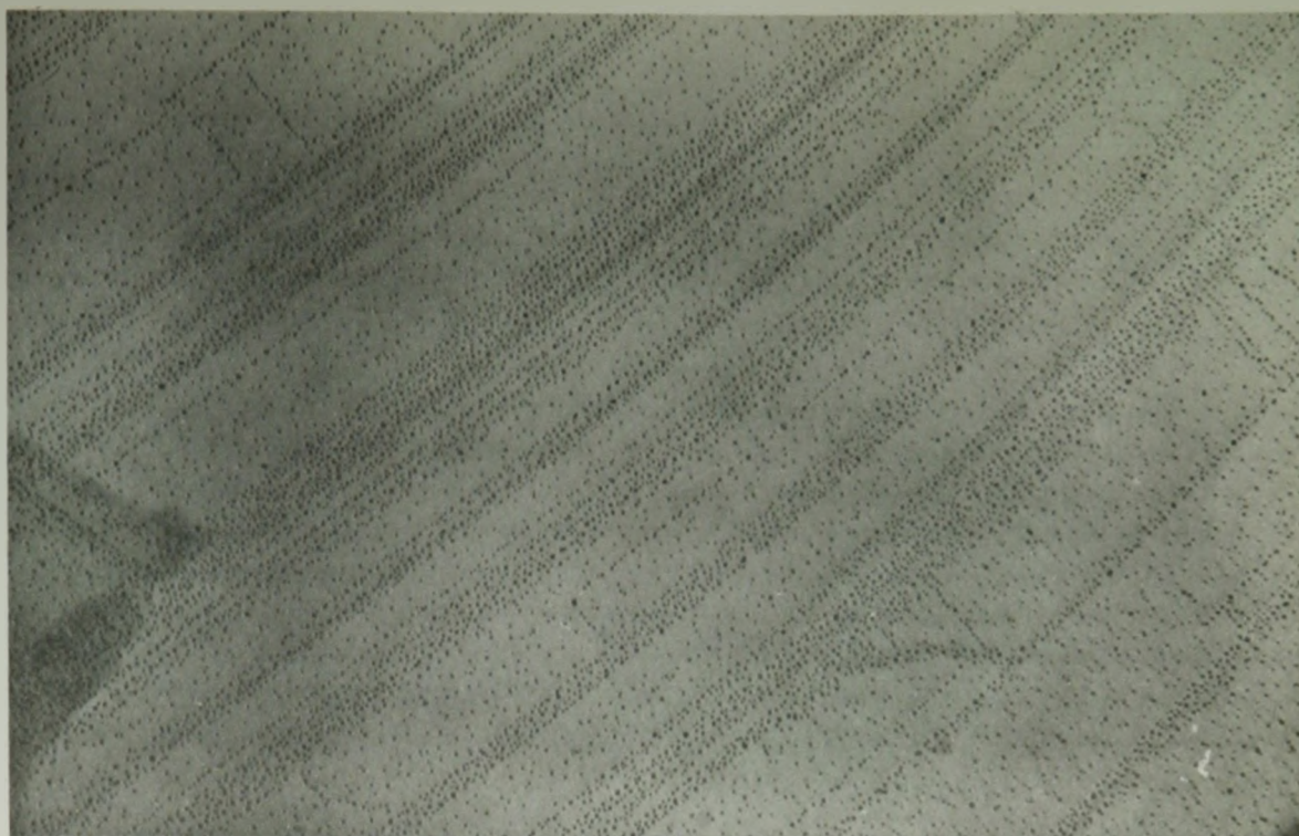
FIGURE 10: Nucleation of gold on cleavage surface of lithium fluoride at 200°C. (110,000 X)
