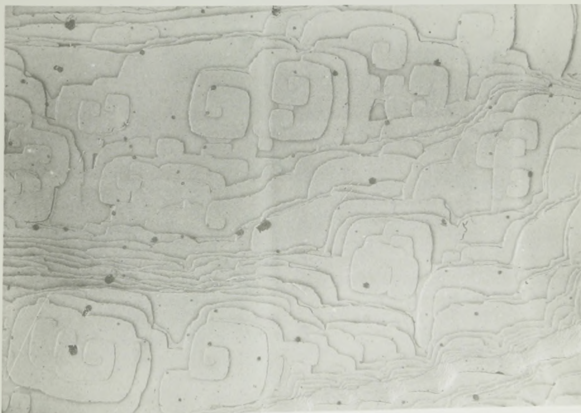
FIGURE 42: Inhibitor concentration 9 p.p.m. Fe Time of etching 10 seconds (16,000 X)
