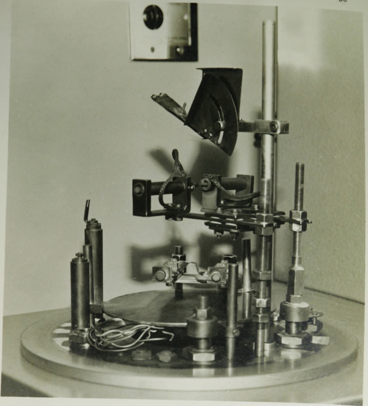
FIGURE 9: Experimental set up for the evaporation of gold and platinum-carbon pellets
