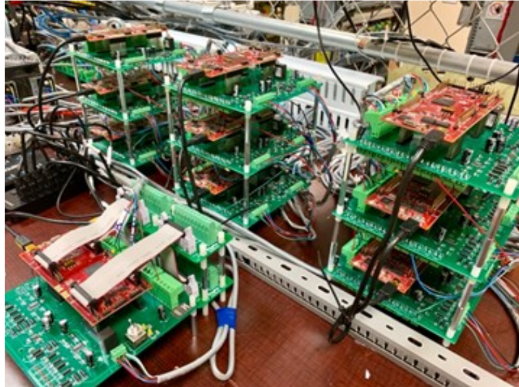
Fig. 3. 29 Cloud DSP System for AFEs
