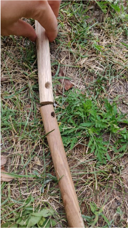
Figure 4.7. Photograph of a space in between each dowel segment used to hold iButtons and separate them at discrete depths in the temperature rods.
