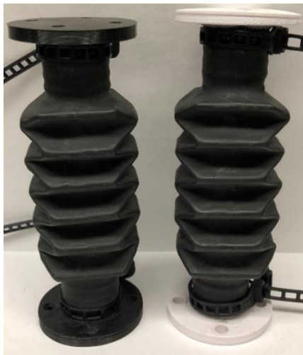
Figure 5.11 The accordion pattern OSPA used for testing. Two fabricated prototypes.
