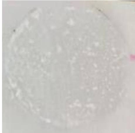
Figure D1. Cation-exchange membrane after 8 hours of ED operation 7.6 \text{ mA/cm}^2 with domestic wastewater dewatering centrate.
