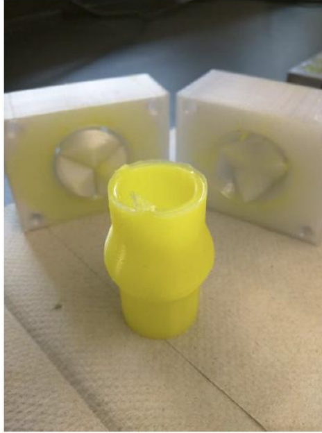
Figure 3.8. Aortic valve model made from Silicone A10 (Si A10) with 3D printed casting mould (PETG material).
