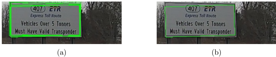
Figure 3.13: Failure case sample caused by candidates selection stage. (a) Extracted candidates (b) Final selected region
