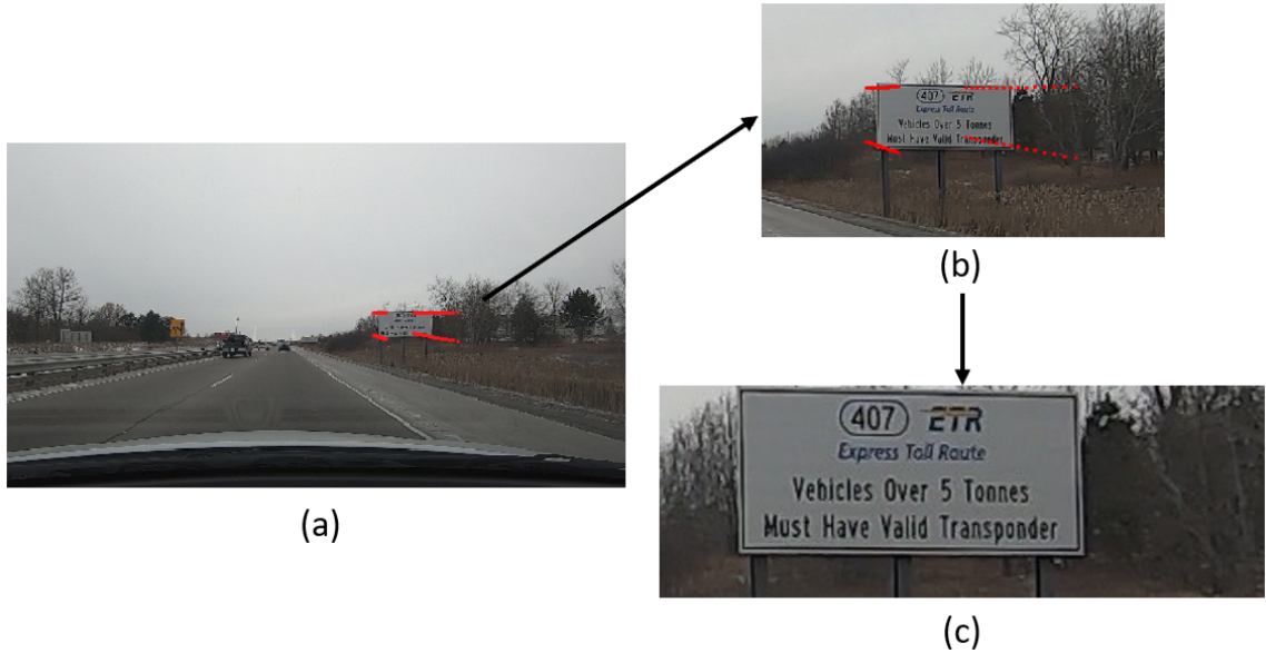
Figure 3.6: The result after the defined search region step. (a) and (b) Predicted corner points in red (c) Final defined search region.
