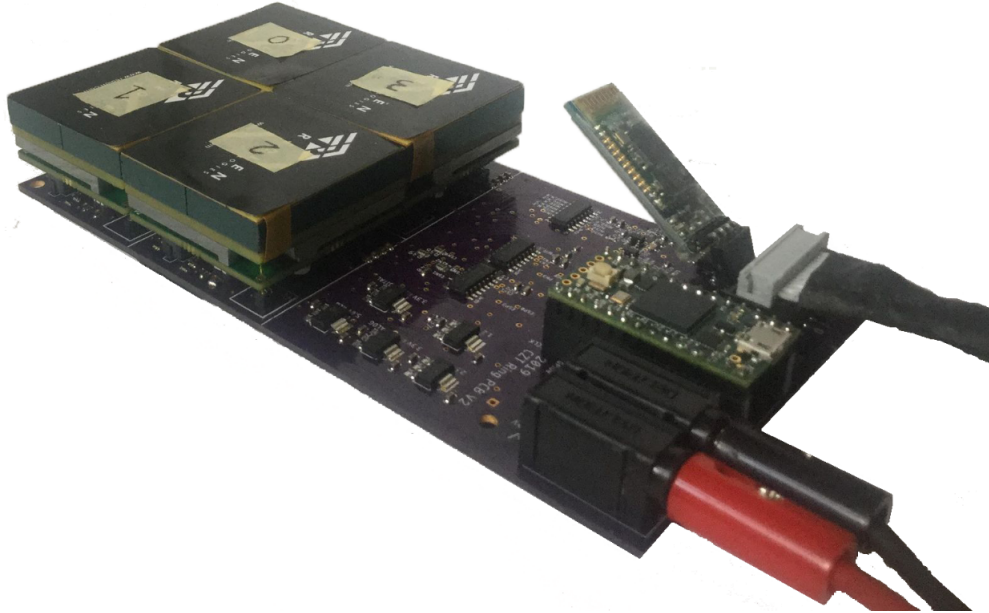
FIGURE 4.1: Single gamma camera module used for testing of mutual interference effects. The camera consists of four CZT detector modules, a PCB, a microcontroller, Bluetooth communication, and high and low voltage supply cables.
