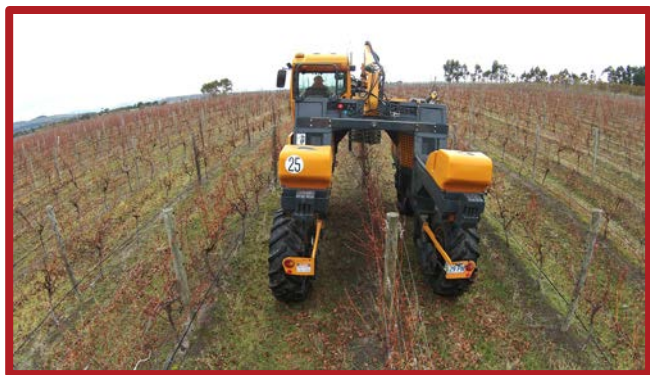
FIGURE 4: MECHANICAL PRUNING. A machine pruning grapevines. The operator decides where to make the cuts and how frequently. Note how the machine functions “over-the-vine” and is capable of fitting through the narrow spaces between rows 10 .
