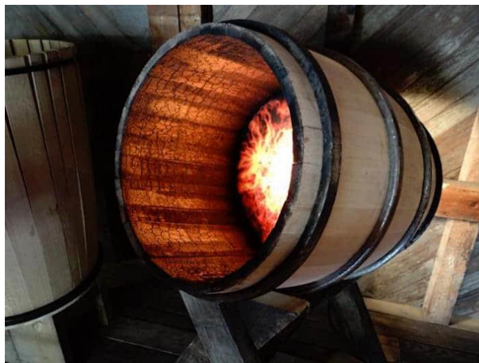
FIGURE 2: OAK BARREL TOASTING. A barrel being treated in the form of toasting. The level of heat and charring will break down the ellagitannins to alternative forms, which will contribute to diverse flavour profiles 6 .
