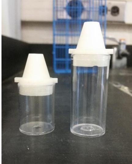
*Figure S3.1: Comparison of vials used in chapter 3 (left) versus chapter 2 (right) with modified funnel cap. Vials used in chapter 3 experiment measured 32mm in height while vials in chapter 2 were 50mm. All other dimensions of the vials were the same*
