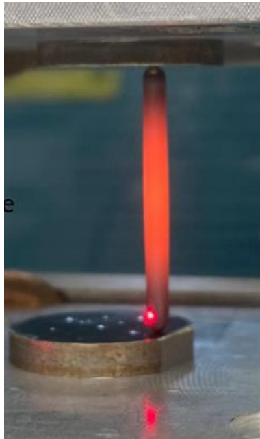
Figure 44: 1.5 mm pin radius glowing.
