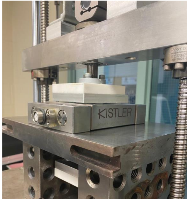
Figure 35: Load-cell setup calibration.
