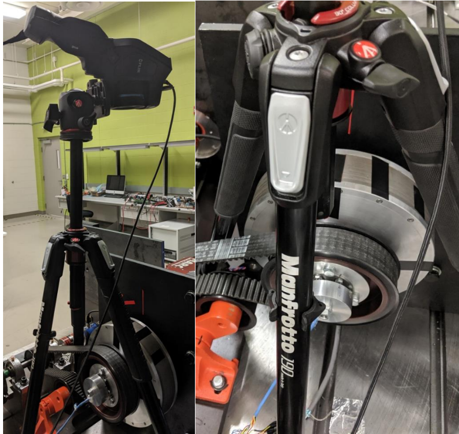
Figure 6-2: Placement of the camera and tripod relative to the motor outer surface
