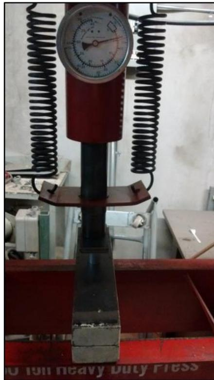
a. Setup for making re-entrant cavities
