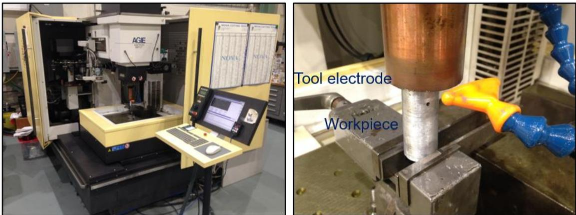
*Figure 3.5: Electrical Discharge machining setup*
