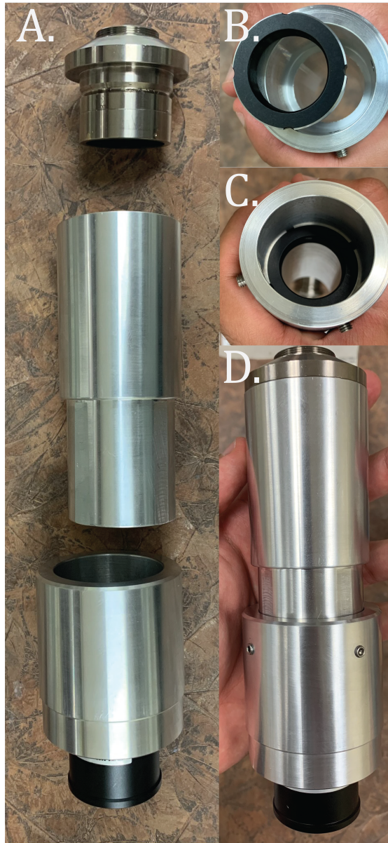
FIGURE 3.9: Tube lens and emission filter holder. A. The three components of the tube lens holder and emission filter holder. The topmost piece is the C-mount which attaches to the camera, the middle piece allows for an adjustable length to accurately place the tube lens away from the camera chip which is held in the last piece. B. and C. A specially made filter holder slides into the tube so that it is placed right where the end of the C-mount is inside the tube. D. Assembled holder.
