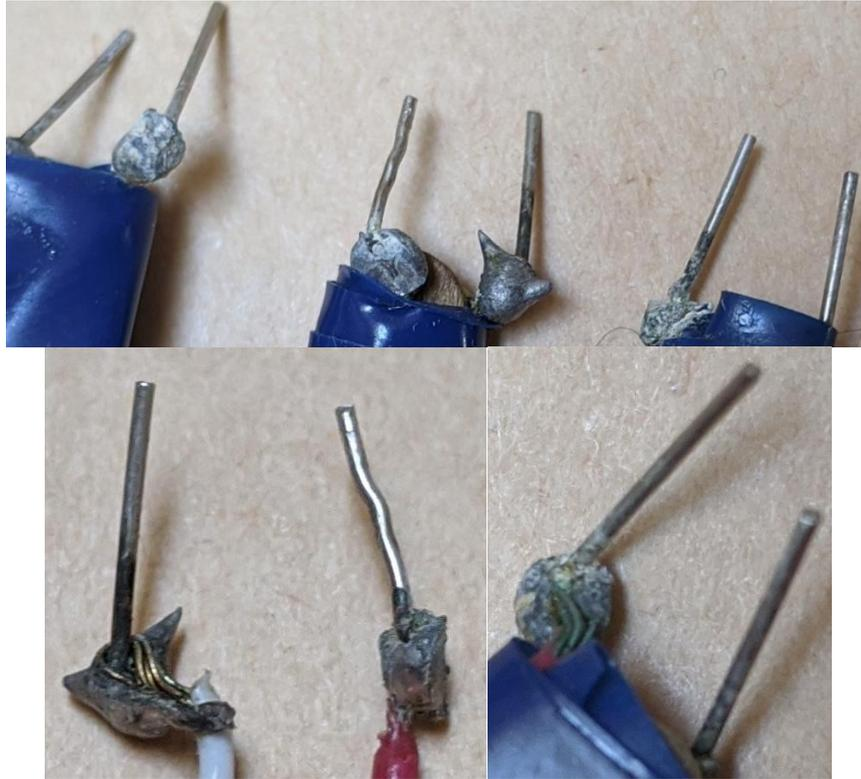
**Figure 6:** Electrode deterioration and precipitate formation
