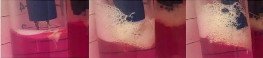
**Figure 12** Electrode gas formation 10 min, 210 Minutes, 420 Minutes
