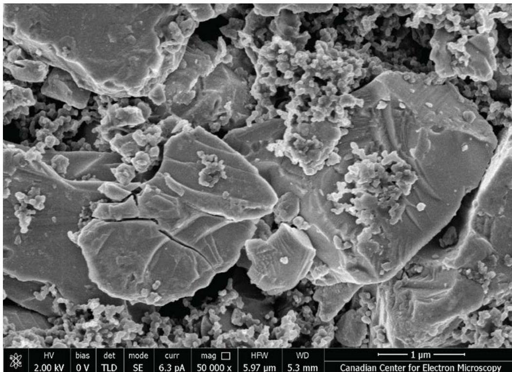
Figure 5.2: SEM image of the pristine silicon anode material revealing micron-sized silicon particles nested in a binder network.
